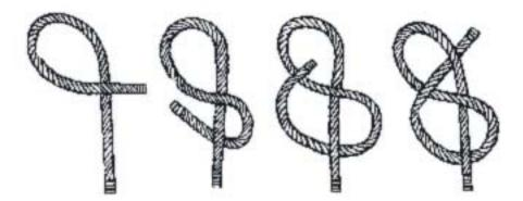
The above diagram shows the figure eight knot. To create a rewoven figure eight, pass the working end through the toggle hole or soft pad eye and then reverse the direction of the line.
