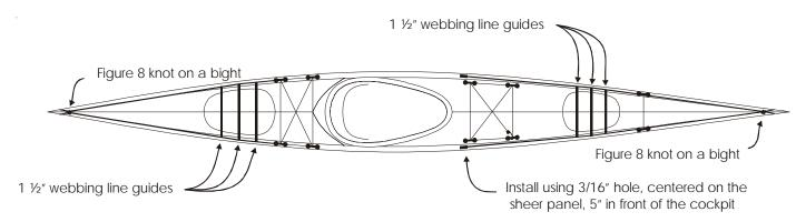
To add a perimeter line to your boat as shown in the diagram, you will first need to create and install two soft pad eyes and line guides made from your hatch straps.
