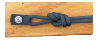
To install the soft pad eyes onto the deck sheer panel, drill a 3/16" hole in the center of the sheer panel, about 5" forward from the front edge of your cockpit opening. This should put the soft pad eye in line with the nylon pad eyes nearest the cockpit opening on your bow deck rigging. Seal the plywood edge of the hole with epoxy and let cure. Then bolt the webbing loop onto the boat.
