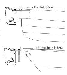
If you are mounting a raked stern bracket, (lower diagram) fore drill first one side of the hull and then the other side of the hull. Screw the self tapping #6 SS sheet metal screws through the bracket into the hull. The short ones are for the rear holes; the longer ones are for the forward holes. Remove the screws and bracket. Fill the holes with epoxy and saturate the end grain exposed by drilling the holes. Re-attach the bracket. Threading the screws into the wet epoxy.
